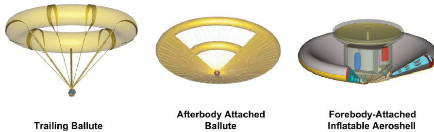
Fig. 1 Inflatable decelerators for aerocapture, from [4].
